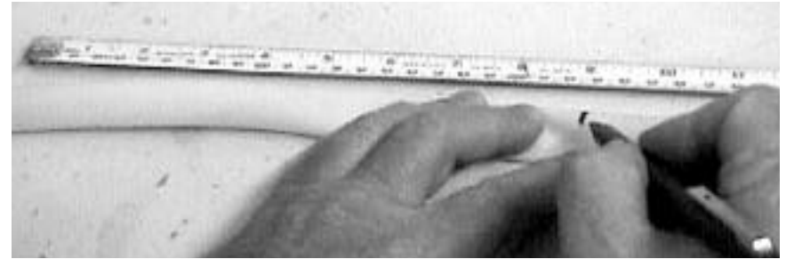
Marking the tube at 8 1/2 inches.
