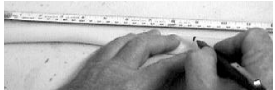
Marking the tube at 9 inches.
