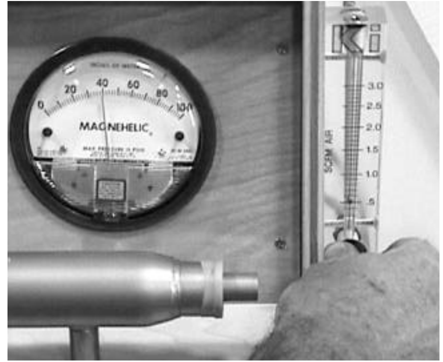
Adjust the knob at the bottom of the Flow Meter.
