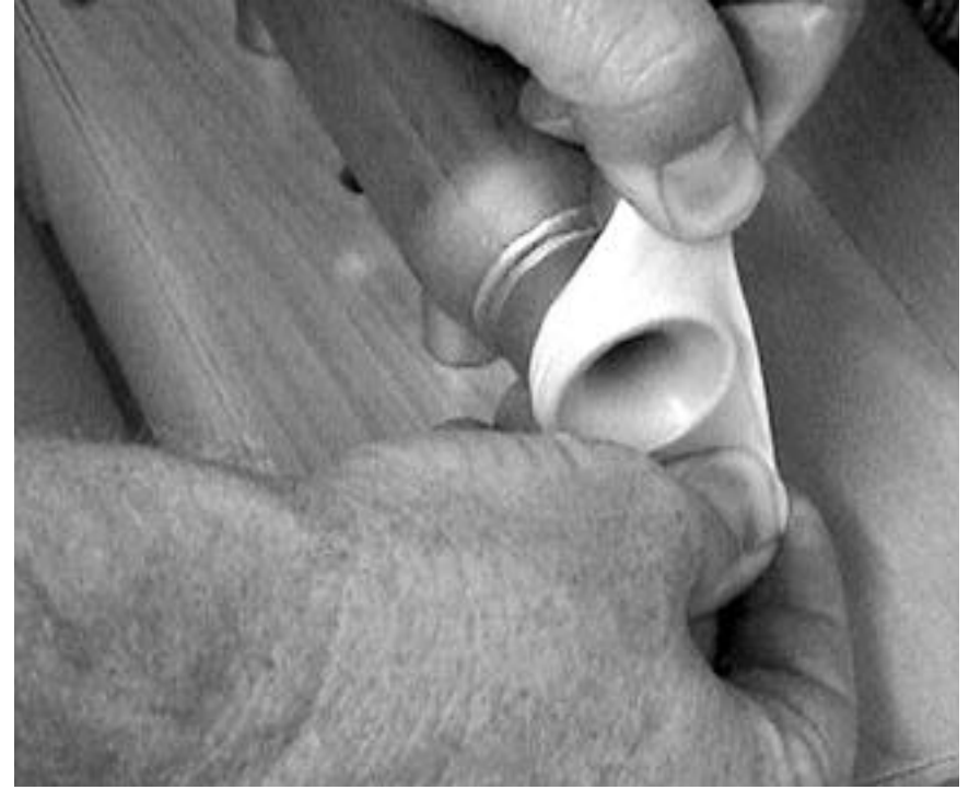
Stretching latex tube over end of Test Chamber.
